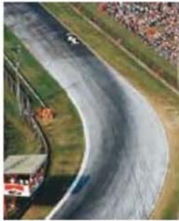
FIGURE 5-22 Race car heading into a curve. From the tire marks we see that most cars experienced a sufficient friction force to give them the needed centripetal acceleration for rounding the curve safely. But, we also see tire tracks of cars on which there was not sufficient force—and which unfortunately followed more nearly straight-line paths.
